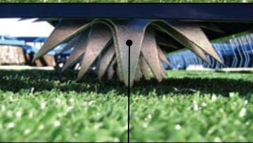
Rotating tines between brushes to perforate and loosen infill
